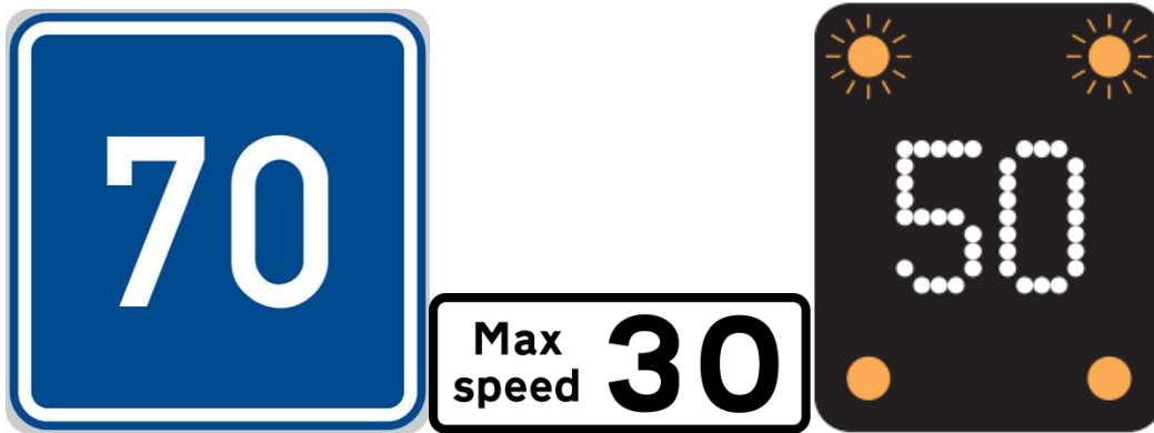
Figure 22: Advisory maximum speed limit signs, in this case fixed signs from the Czech Republic (L) (By Frisky007 - Own work, CC BY-SA 3.0, https://commons.wikimedia.org/w/index.php?curid=10803559 ) and the UK (C) (By UK Government - UK Traffic signs image database, Public Domain, https://commons.wikimedia.org/w/index.php?curid=17332626 ) and a temporarily activated LED sign from the UK (R) (You may re-use this information (not including logos or third-party material) free of charge in any format or medium, under the terms of the Open Government Licence v2.0. To view this licence, visit www.nationalarchives.gov.uk/doc/open-government-licence/version/3 or write to the Information Policy Team, The National Archives, Kew, London TW9 4DU, or e-mail: psi@nationalarchives.gsi.gov.uk )
