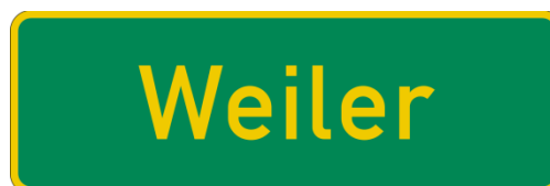
Figure 14: An example of a German place name sign, that is intended to mark the entrance to a town or village, without implying a change in speed limit for that road. (By Andreas 06; new drawing: Mediatus - de:Strassenverkehrs-Ordnung (German Road Regulations) 1992, Verkehrsblatt, DIN-Normen, Public Domain, https://commons.wikimedia.org/w/index.php?curid=1005489 )
