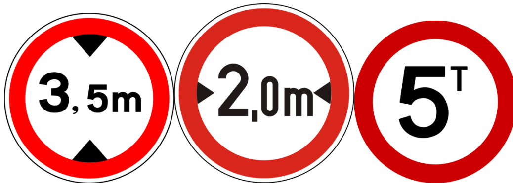
Figure 20: Numerical limit signs, that have the potential to be confused with speed limit signs, indicating maximum values for vehicle height (L) (By Gigillo83 - Own work, CC BY-SA 4.0, https://commons.wikimedia.org/w/index.php?curid=38690556 ) width (C) (By Gigillo83 - KRESZThe Hungarian Highway Code, Public Domain, https://commons.wikimedia.org/w/index.php?curid=31680336 ) and Weight (R) (By Peeperman - Own work, Public Domain, https://commons.wikimedia.org/w/index.php?curid=10125764 )
